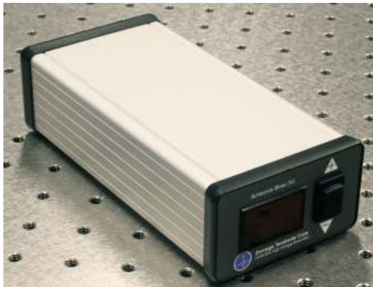
Figure 33: High voltage modulator for photoconductive antenna [59].
