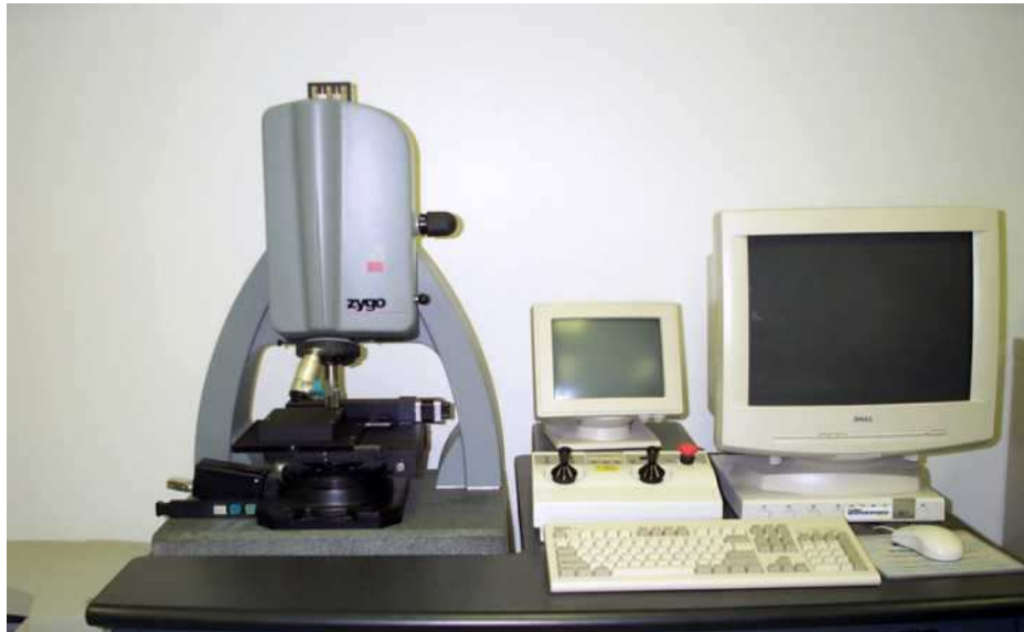
Figure 83. Zygo scanning white light interferometer.
