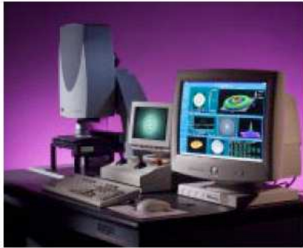
Figure 84. Zygo Micro-LUPI phase-shifting interferometer [56].
