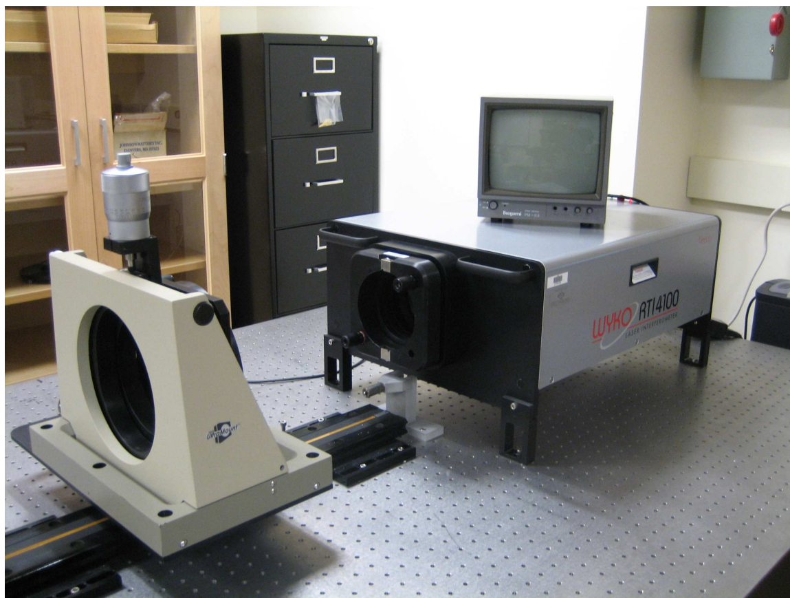
Figure 82. Wyko RTI 4100 laser Fizeau interferometer.
