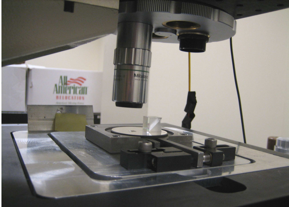
Figure 31. Optical flat assembly on microscope stage.
