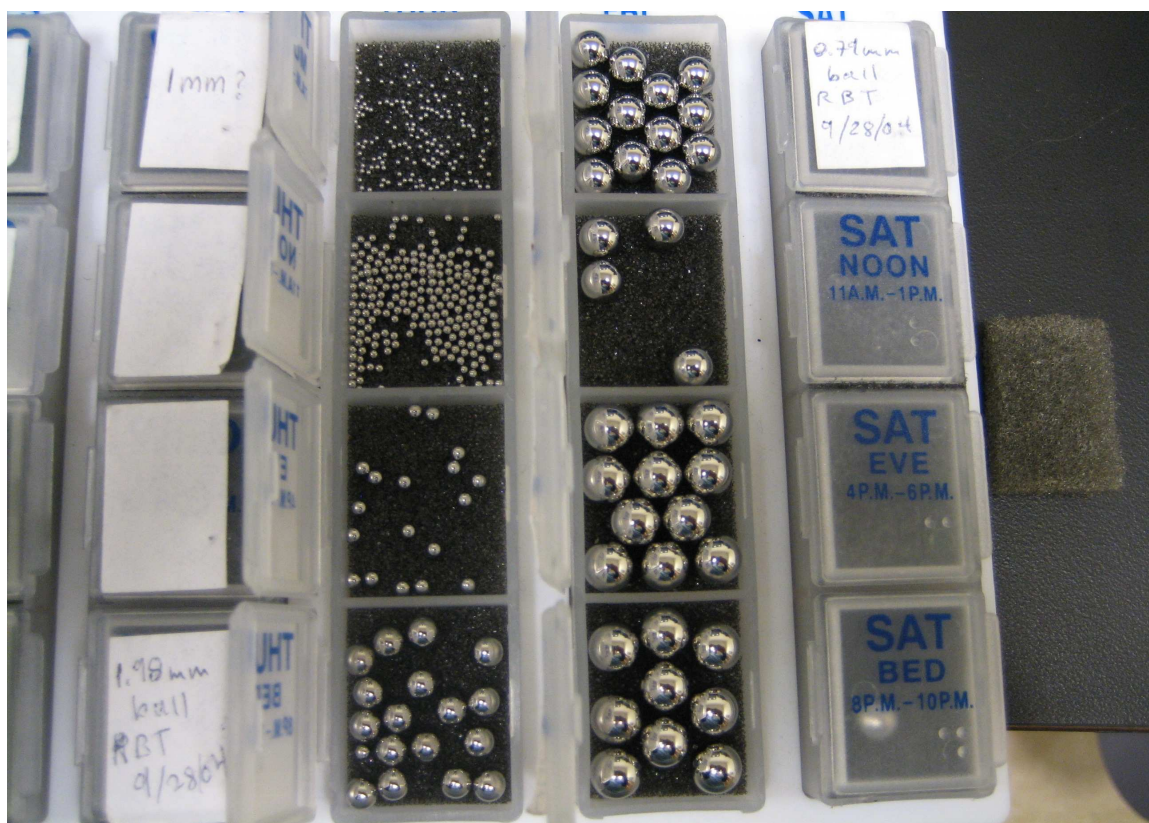
Figure 61. 440-steel micro-spheres; radii 0.5 – 3 mm [52].
