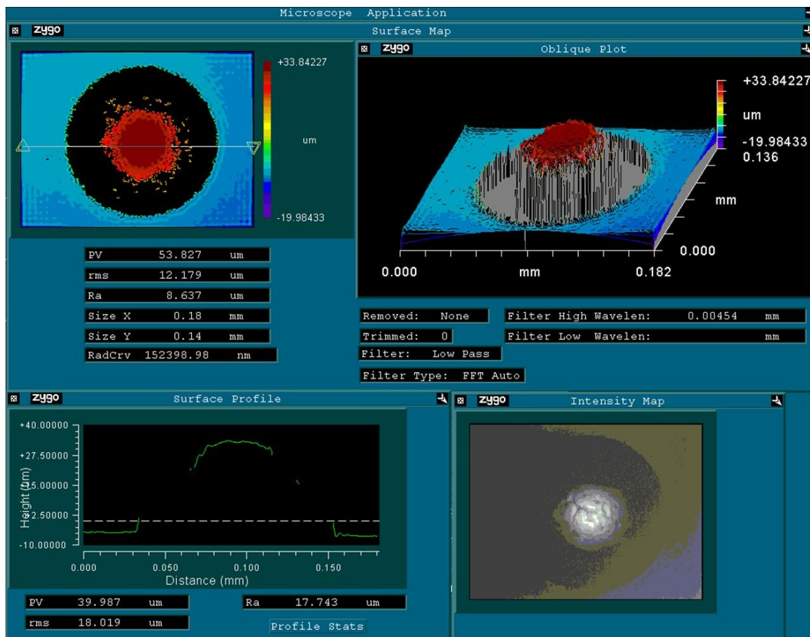
Figure 5-9. A snapshot of the MetroPro™ screen showing the measurement results. The top-left image is the 2-D height map where different height values are presented by different colors. Underneath is a 2-D cross sectional profile across the line shown at the middle of the top-left image. The top right image is the 3-D map of the bump, and underneath it is a gray-scale intensity map.
