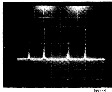
Fig. 2 Optical spectrum of light analysed by scanning CFP
