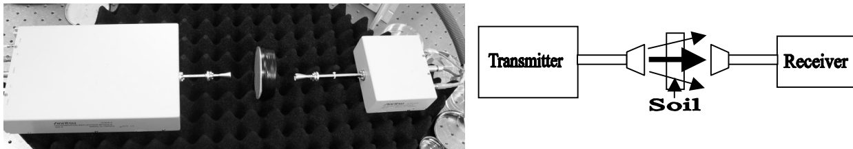
Figure 2: Photograph (Left) and schematic (Right) of the vector network analyzer's transmitter and receiver equipped with horn antennas in the transmission configuration.
