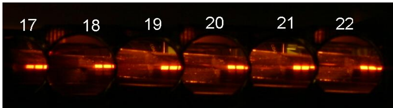
Figure 6. Several of the imaged slitlets with a scene consisting of a set of illuminated cross-slice slits. As expected, only approximately one half of each slitlet shows the illuminated slits, with the other half being dark.
