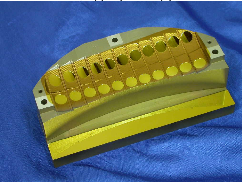
Figure 5. The monolithic imaging mirror assembly (gold-plated and overcoated aluminum). The 22 spherical mirror surfaces have different tilt angles and radii of curvature, but are diamond turned into a single monolithic substrate.
