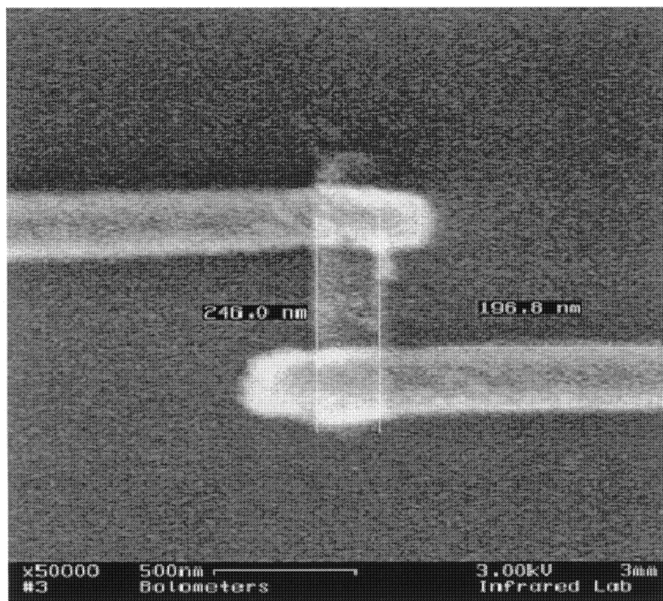
Figure 2. First set of antenna-coupled microbolometers fabricated using Aluminum for the dipole antenna arms.
