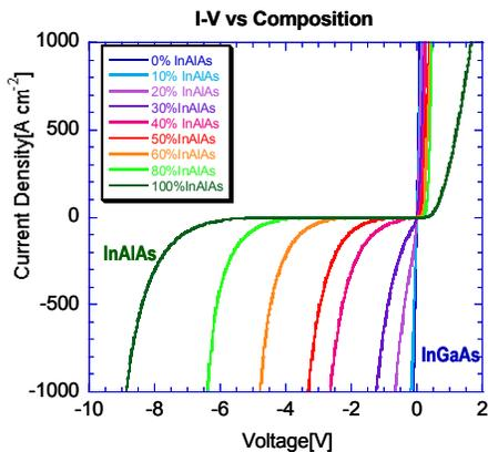
Figure 2 – Digital alloy performance control on the S<sup>3</sup> detectors using semimetal-semiconductor interfaces
