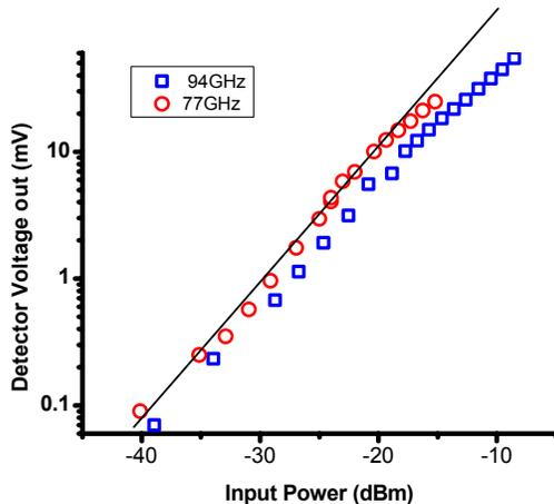
Figure 7- S3 Detector output voltage as a function of detector power input
