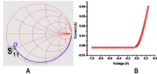
Figure 3- Smith chart data from dc-110GHz and the I-V characteristics of the S3 detectors
