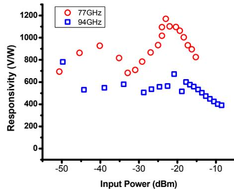
**Figure 6- S3 Detector Responsivity as a function of detector input power at 94 and 77GHz**
