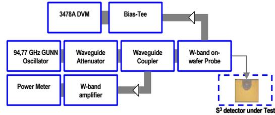
**Figure 5- W-band Reflectometer setup for responsivity measurements of the S<sup>3</sup> detector**
