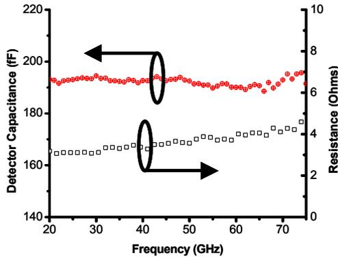
**Figure 4- Device capacitance and resistance as a function of frequency for the 20 $\mu$ m Semimetal Semiconductor Schottky Detector**
