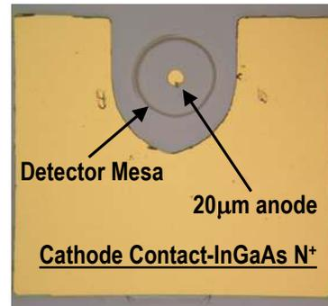
Figure 1- The  $S^3$  detector geometry for MMW characterization
