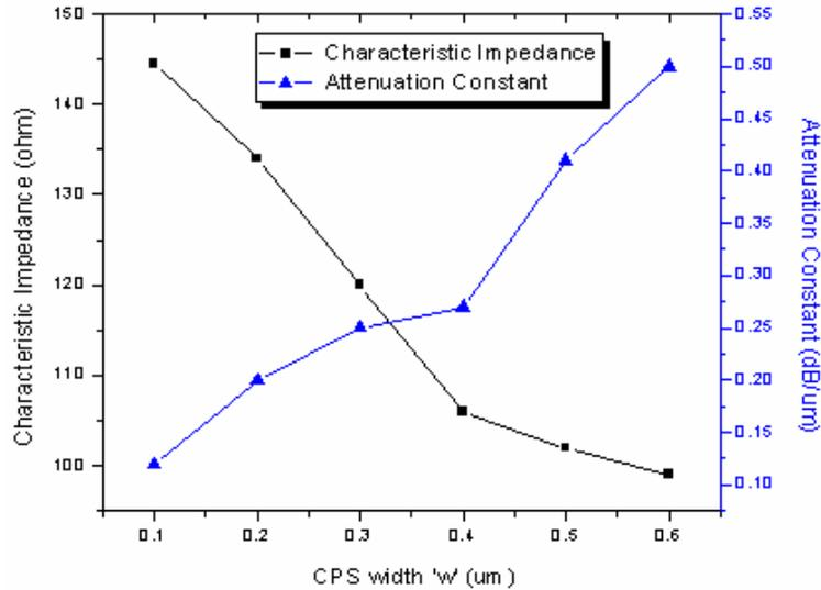
**Figure 2**  $Z_0$  and  $\alpha$  for CPS separation of 0.4- $\mu\text{m}$
