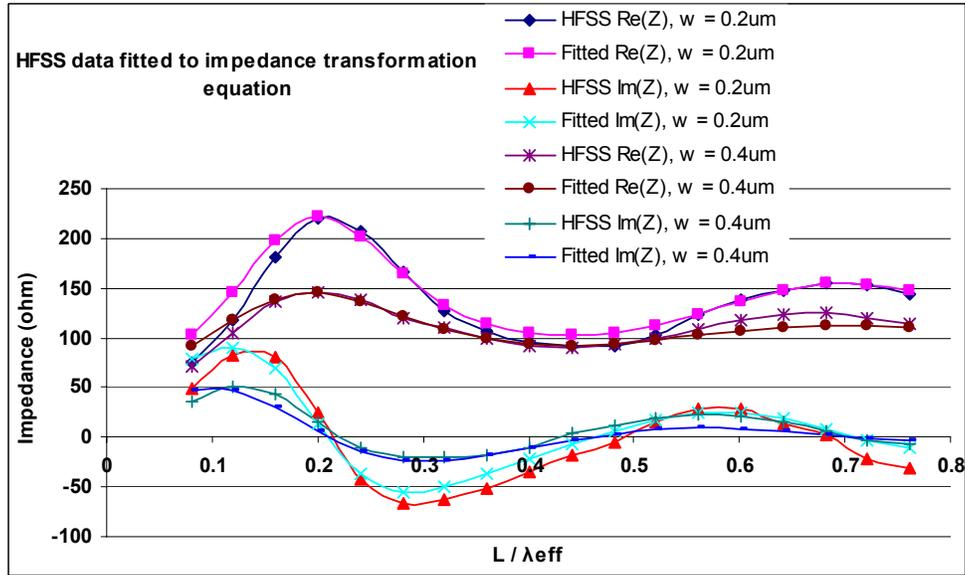
**Figure 1** Curve fitting of HFSS data to eq. (2) for  $w = 0.2\text{-}\mu\text{m}$  and  $0.4\text{-}\mu\text{m}$
