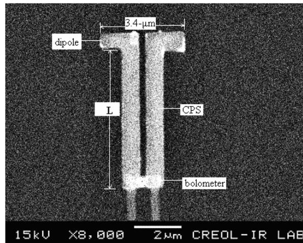
**Figure 3** Dipole antenna connected to CPS
