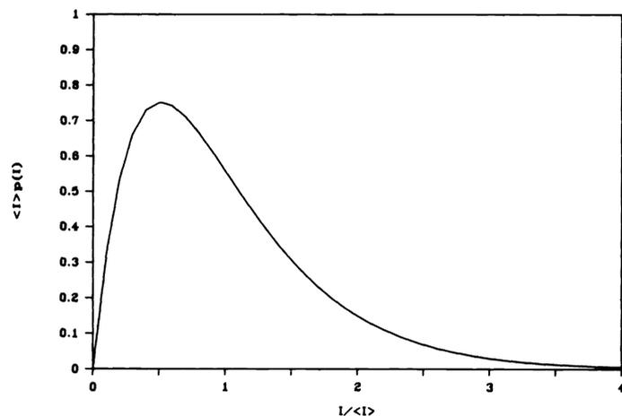
Fig. 5. Normalized speckle PDF calculated from Eqs. (1) and (2).
