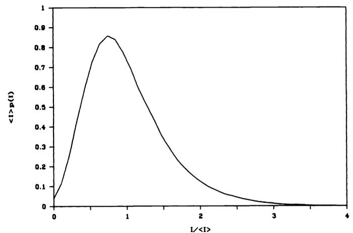
Fig. 3. Normalized speckle PDF measured inside the shadow region.
