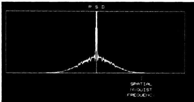
Fig. 7. PSD measured for speckle outside the shadow region. The arrow indicates the spatial Nyquist frequency of 21.5 cycles/mm.
