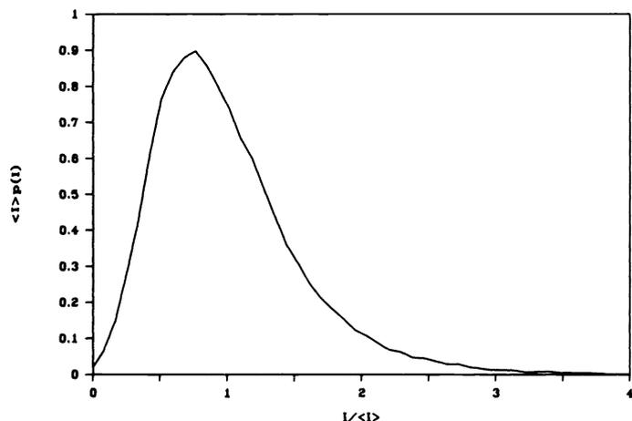
Fig. 4. Normalized speckle PDF measured outside the shadow region.
