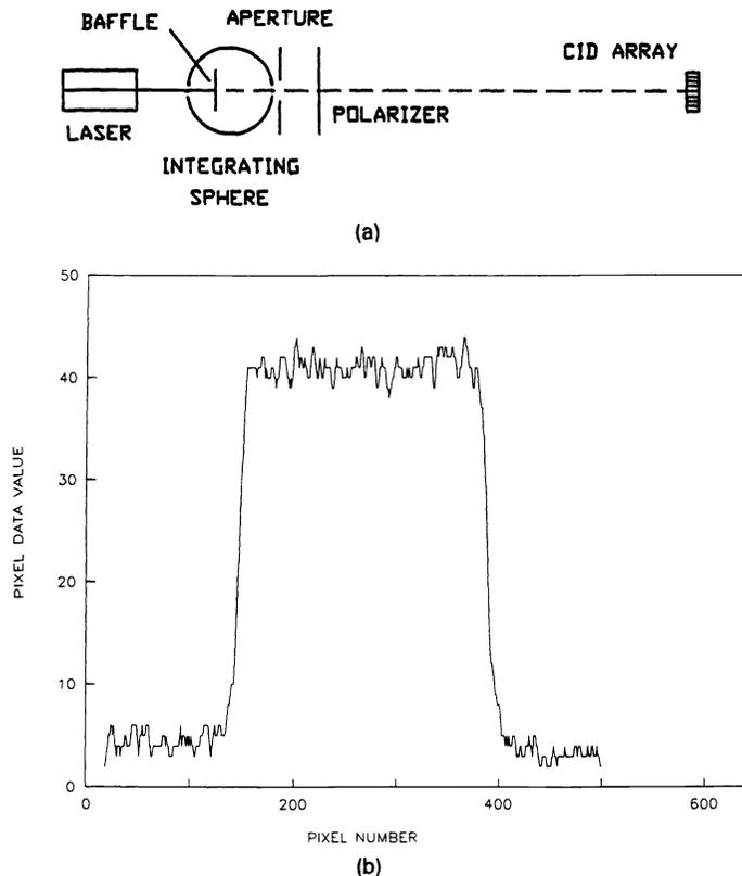
Fig. 1. (a) Experimental setup used for the production of speckle patterns. (b) Profile of irradiance vs position for an image of the output aperture of the integrating sphere.
