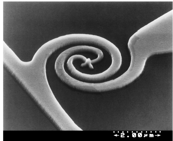
Fig. 1. Electron micrograph of a Ni–NiO–Ni diode with an integrated asymmetric spiral antenna.
