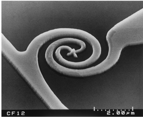
Fig. 1. Electron micrograph of a spiral antenna from the air side.
