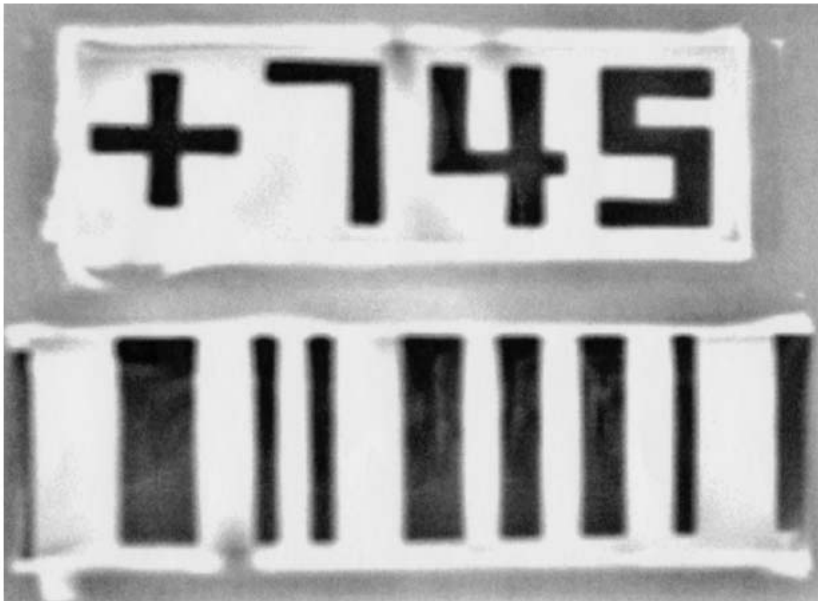
Figure 3. The thin film barcode in the infrared, taken with a Raytheon ControlIR 2000B camera, equipped with optics that view from 8 to 12 \mu m.
