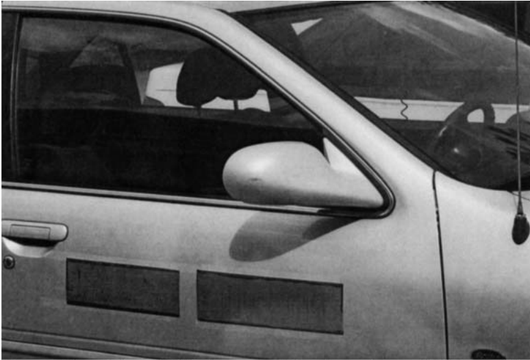
Figure 6. The visible image of the barcode application. The barcode forms to the contours of the automobile's door and blends with its metallic color.
