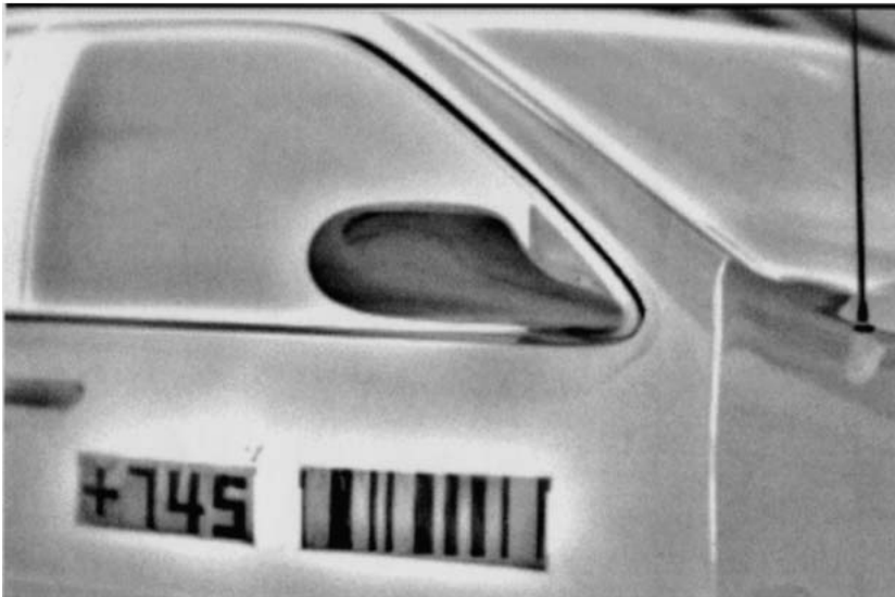
Figure 5. An application of the thin film barcodes. The infrared image is taken with radiation from 8 to 12 \mu m. This automobile was allowed to sit in the sun and barcode contrast was enhanced.
