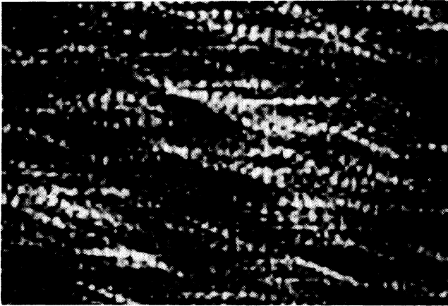
Fig. 9 Representative speckle pattern obtained with the extended-frequency aperture.
