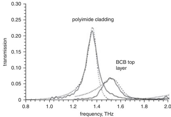
**Fig. 3** Top cladding for type 2 gangbuster replaced with BCB and compared to all polyimide cladding
