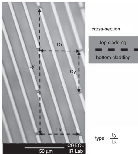
**Fig. 1** Dipole metamaterial array configuration indicating gangbuster type with cross-section shown on right where thicknesses of top and bottom cladding layers are typically 9 μm and metal elements in centre are approximately 200 nm
