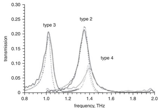
**Fig. 2** Transmission for gangbuster type 2, 3, 4 with linearly polarised input. Measured data, solid lines; model predictions, broken lines
