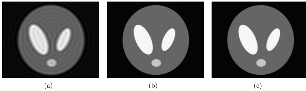
Figure 7. Images of the phase object reconstructed from noiseless data by use of the (a) single-plane, (b) half-scan and (c) conventional I-DT reconstruction algorithms. The scanning geometries corresponded to the values \lambda = 1 \times 10^{-3} , d = 0.4 and \Delta = 0.05 .
