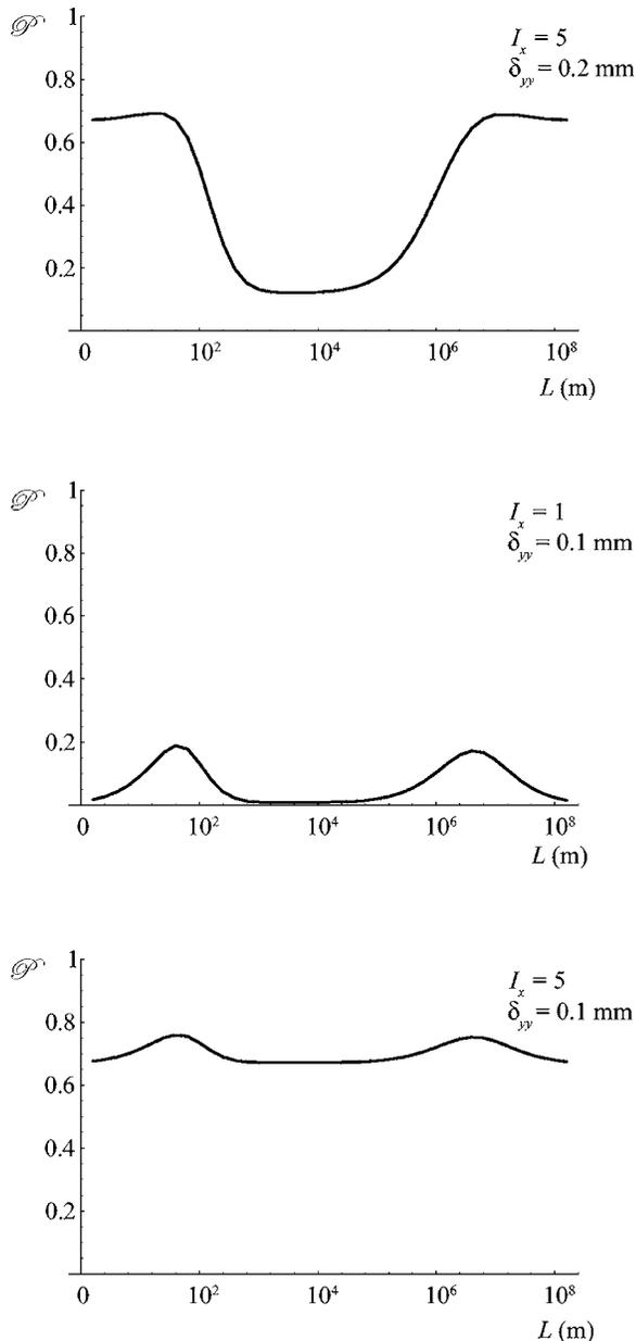
Fig. 6. On-axis degree of polarization of a beam of mixed-correlation type as a function of propagation distance  $L$  for different values of spatial coherence and source degree of polarization. In all cases,  $I_y=1$ ,  $\delta_{xx}=0.1$  mm,  $\sigma_l=5$  cm, and  $C_n^2=10^{-14}$  m $^{-2/3}$ .
