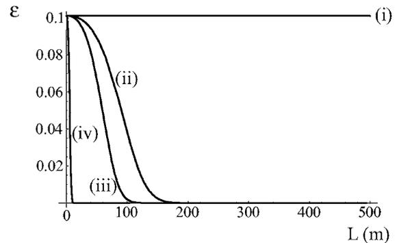
Fig. 3. Evolution of the degree of polarization for a pair of tilted, partially correlated plane waves with  $I_1=1$ ,  $I_2=2$ , and  $\mu=0.5 \exp[i\pi/4]$ . Here (i) represents  $\Delta k=0$ , (ii) represents  $\Delta k=0.001k$ , (iii) represents  $\Delta k=0.002k$ , and (iv) represents  $\Delta k=0.1k$ . All other parameters are as in Fig. 2.
