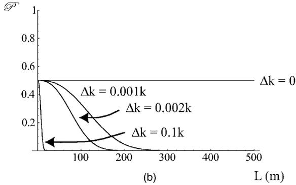
Fig. 2. Evolution of the degree of polarization for a pair of tilted, partially correlated plane waves of equal intensity. (a)  $\mu=1$ ; (b)  $\mu=0.5$ . Here  $\lambda=1 \mu\text{m}$ ,  $C_n^2=10^{-14} \text{m}^{-2/3}$ , and  $\Delta k=k|\mathbf{u}_2-\mathbf{u}_1|$ .
