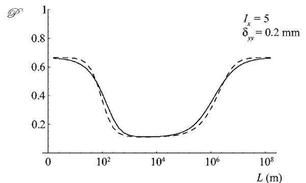
Fig. 4. On-axis degree of polarization of a Gaussian Schell-model beam as a function of propagation distance  $L$  for different values of spatial coherence and source degree of polarization. In all cases,  $I_y=1$ ,  $\delta_{xx}=0.1$  mm,  $\sigma_l=5$  cm, and  $C_n^2=10^{-14}$  m $^{-2/3}$ .
