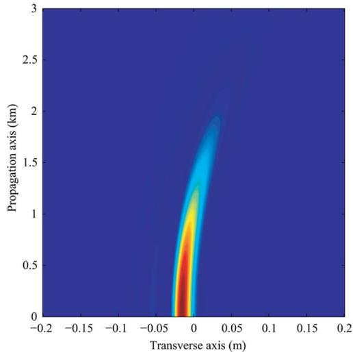
Fig. 2. (Color online) Illustration of the average propagation dynamics of an Airy beam as a function of distance on propagation in turbulence. The transverse axis is the  $45^\circ$  axis in the  $x$ - $y$  plane. The parameters are the same as in Fig. 1.
