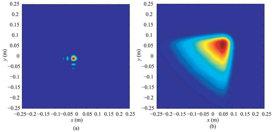
Fig. 1. (Color online) Illustration of the intensity patterns of an Airy beam in the (a) transmitter plane and (b) receiver plane. The wavelength is  $\lambda = 1.55 \mu\text{m}$ , the turbulence strength is  $C_n^2 = 10^{-14} \text{ m}^{-2/3}$ , and the propagation distance is  $L = 3 \text{ km}$ .
