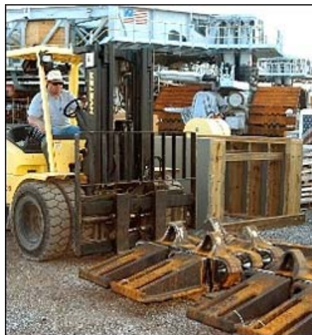
New crawler shoes arrive at KSC in truckloads of 20 to comply with shipping-load limits. One of NASA's two crawlers is in the background. NASA [larger image]
