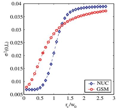
Fig. 1. On-axis scintillation index  $\sigma^2(0, L)$  of an NUC beam and a GSM beam as a function of  $r_c/w_0$ . Here,  $\lambda = 1.55 \mu\text{m}$ ,  $L = 2 \text{ km}$  and  $w_0 = 0.05 \text{ m}$ .
