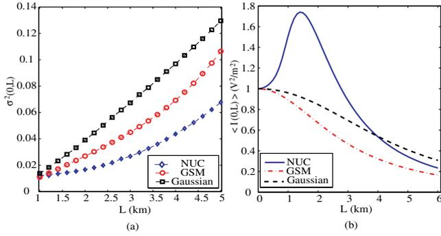
Fig. 2. (a) On-axis scintillation index  $\sigma^2(0, L)$  and (b) On-axis average intensity  $\langle I(0, L) \rangle$  of an NUC, a GSM, and a coherent Gaussian beam as a function of the propagation distance  $L$ . Here,  $r_c = 0.91w_0$ .
