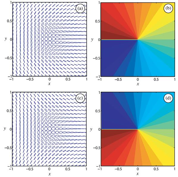
**Fig. 1.** Illustration of the state of polarization around (a), (b) a lemon and (c), (d) a star. Blue represents  $\theta = -\pi/2$ , while red represents  $\theta = +\pi/2$ .
