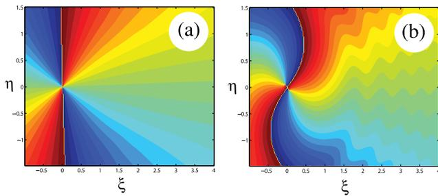
**Fig. 4.** Polarization of the field for (a) the radial polarization element at  $\alpha = 0.99$  and (b) the lemon polarization element at  $\alpha = 1.99$ .
