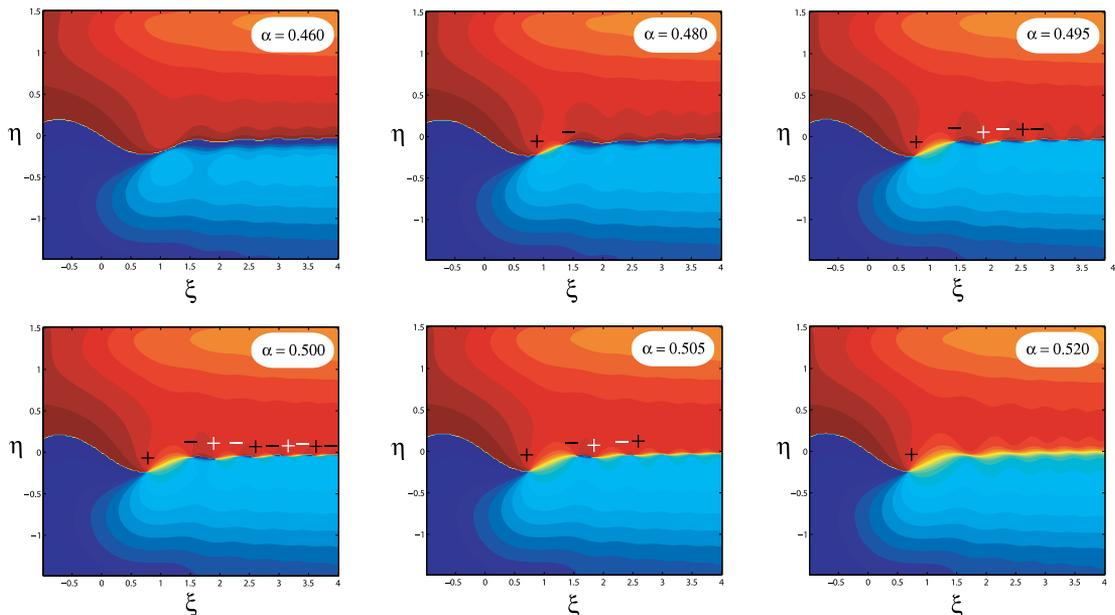
**Fig. 3.** Illustration of the evolution of the polarization singularities as a function of  $\alpha$ . Here  $\xi = x\sqrt{k/4z}$  and  $\eta = y\sqrt{k/4z}$ .
