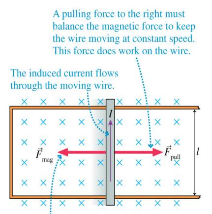
Mechanical \_ Power:  $P_{input} = F_{pull}v = \frac{v^2 l^2 B^2}{R}$ Electrical \_ Power:  $P_{dissipated} = I^2 R = \frac{v^2 l^2 B^2}{R}$
