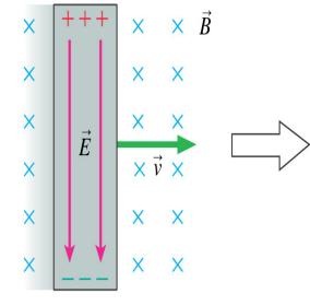
charge separation creates an electric field in conductor.  $\vec{E}$  increases as more charge flows.
