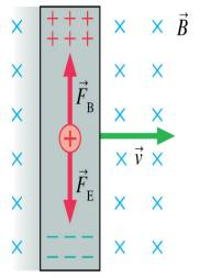
The charge flow continues until the downward electric force  $\vec{F}_{\rm E}$  is large enough to balance the upward magnetic force  $\vec{F}_{\rm B}$ . Then the net force on a charge is zero and the current ceases.
