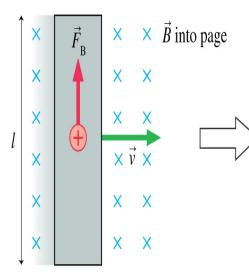
Charge carriers in the wire experience an upward force of magnitude  $F_{\rm B} = qvB$ . Being free to move, positive charges flow upward (or, if you prefer, negative charges downward).
