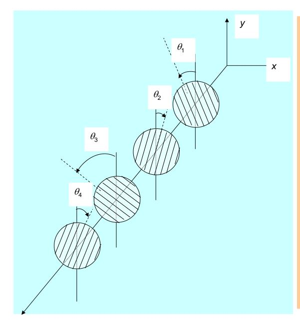
In figure, initially unpolarized light is sent through four polarizing sheets. The first and third sheets have polarizing directions making angles of  $\theta_1$ = 30<sup>°</sup> and  $\theta_3$  = 60<sup>°</sup> (measured counterclockwise) with the direction of the y-axis. The second and forth sheets have polarizing direction making angles of  $\theta_2 = 15^\circ$  and  $\theta_4 = 25^\circ$ (clockwise) with the direction of the y-axis.
