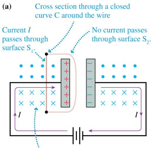
This is the magnetic field of the current *I* that is charging the capacitor.
