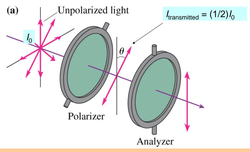
• If incident light is unpolarized the intensity of the beam transmitted through the polarized is  $I_0/2$ .
