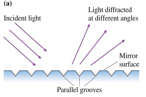
A reflection grating can be made by cutting parallel grooves in a mirror surface. These can be very precise, for scientific use, or mass produced in plastic.
