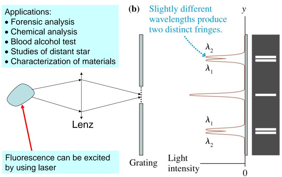
The resolution of the spectrometers is determined by the width of the fringes
