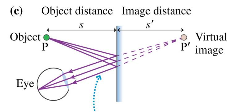
The reflected rays *all* diverge from P', which appears to be the source of the reflected rays. Your eye collects the bundle of diverging rays and "sees" the light coming from P'.
