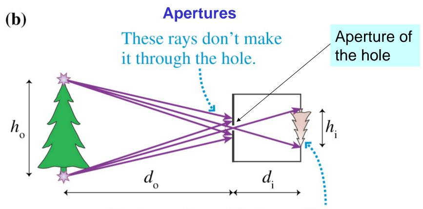
The image is upside down. If the hole is sufficiently small, each point on the image corresponds to one point on the object.
