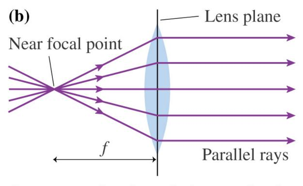
Any ray passing through the near focal point emerges from the lens parallel to the optical axis.
