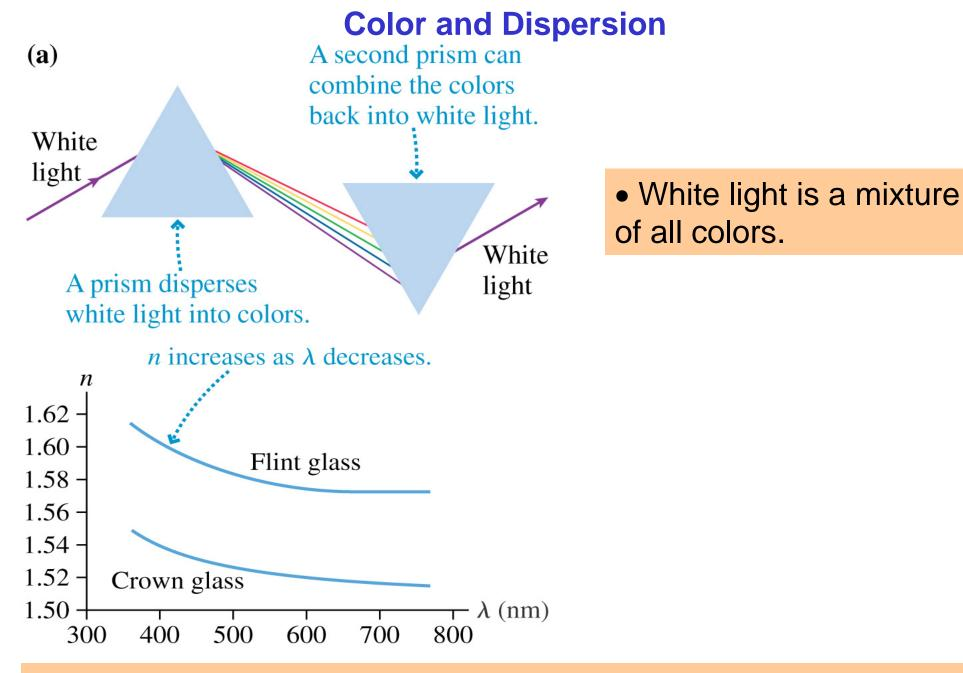
• The index of refraction of a glass differs for different colors.
