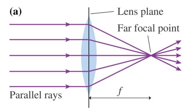
Any ray initially parallel to the optical axis will refract through the focal point on the far side of the lens.
