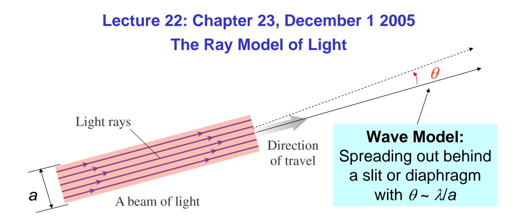
• The ray model of light is valid as long as any apertures through which the light passes (lenses, mirrors, holes, etc.) are very large compared to  $\lambda \Rightarrow \theta \sim 0$ .
