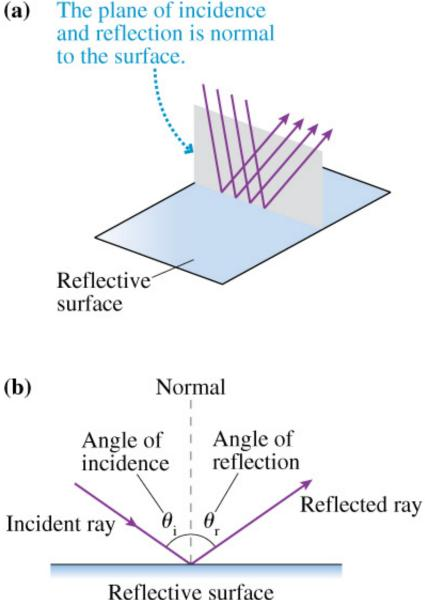
• The incident ray and the reflected ray are in the same plane normal to the surface
