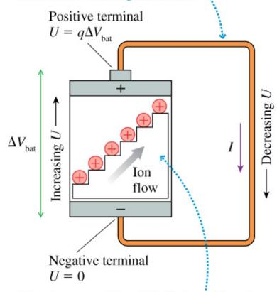
The charge escalator "lifts" charge from the negative side to the positive side. Charge q gains energy  $\Delta U = q \Delta V_{\text{bat}}$ .
