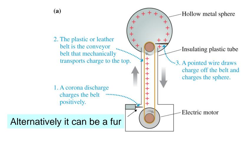
Which forces provide charge separation?
