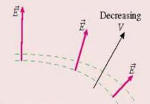
Is inversely proportional to the spacing Δs between the equipotential surfaces.
