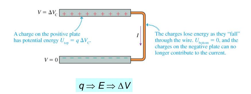
A charged capacitor is a source of potential difference, but it cannot sustain a current
