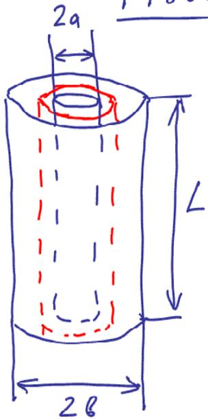
Derive an expression for the capacitance of the cylindrical capacitor in terms of  $a$ ,  $b$ ,  $L$  and  $\epsilon_0$ .
