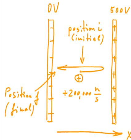
A proton is fired with  $v = 2.0 \times 10^5 \frac{m}{s}$  from the mid point of a capacitor towards the + plate.
