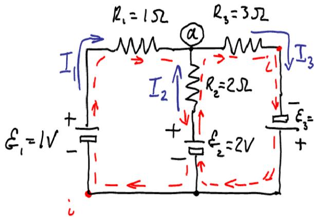
Find the currents  $I_1$ ,  $I_2$  and  $I_3$  in each resistor using Kirchoff's Law
