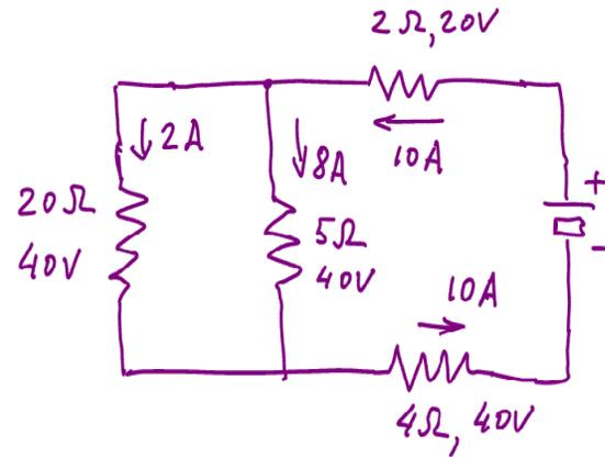
Two resistors,  $20\Omega$  and  $5\Omega$ , must have the same potential difference  $\Delta V = \Delta V_4(\text{left}) = 40V$
