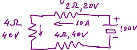
$$\begin{aligned} \Delta V_2 &= (10A) \cdot (2\Omega) = 20V \\ \Delta V_4(\text{left}) &= (10A) \cdot (4\Omega) = 40V \\ \Delta V_4(\text{right}) &= (10A) \cdot (4\Omega) = 40V \end{aligned}$$
