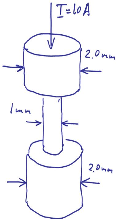
An Al wire consists of the three segments shown in figure. The current in the top segment is 10 A. For each of these three segments, find:
