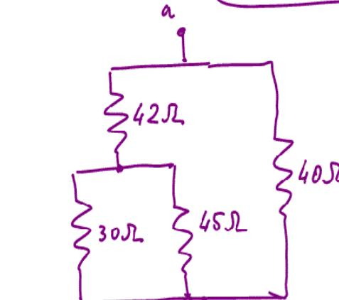
What is the equivalent resistance between points "a" and "b" in Figure?
