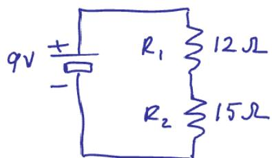
How much power is dissipated by each resistor in Figure?
