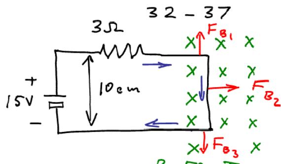
The right edge of the circuit in Figure extends into  $50 \text{ mT}$  uniform  $\vec{B}$ .
