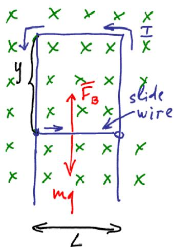
U-shaped conducting rail is oriented vertically in a horizontal  $\vec{B}$ . The rail has no electric resistance and does not move. A slide wire with mass  $m$  and resistance  $R$  can slide up and down without friction while maintaining el. contact with the rail.
