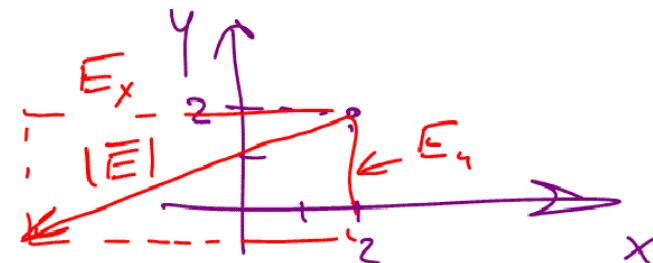
$$\begin{aligned} |\bar{E}| &= \sqrt{E_x^2 + E_y^2} = \sqrt{20^2 + 8^2} = \\ |a| &= \frac{F}{m} = \frac{q \cdot |\bar{E}|}{m} = \frac{21.5 \times 10^{-9}}{10^{-3}} = \\ &= \underline{\underline{21.5 \times 10^{-6} \left[ \frac{\text{m}}{\text{s}^2} \right]}} \end{aligned}$$
