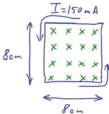
The resistance of the loop is  $0.15\Omega$ . Is the magnetic field strength increasing or decreasing? At what rate ( $\frac{I}{s}$ )?
