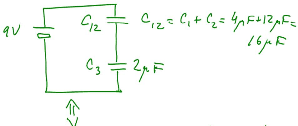
$$\begin{aligned}\frac{1}{C_{123}} &= \frac{1}{C_{12}} + \frac{1}{C_3} = \\ &= \frac{1}{16} + \frac{1}{2} = \frac{1+8}{16} = \\ &= \frac{9}{16}\end{aligned}$$
