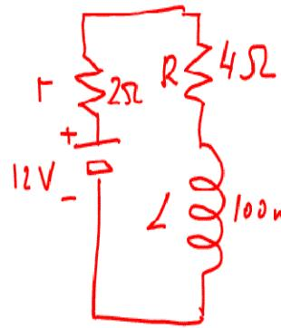
A 100mH inductor whose windings have a resistance of  $4\Omega$  is connected across a 12V battery having an internal resistance of  $2\Omega$ .
