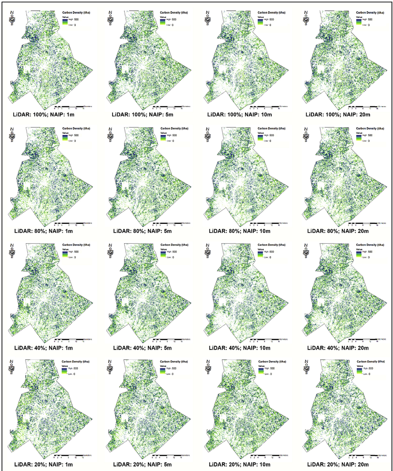
Fig. 3. Forest carbon maps derived from four resolutions (1, 5, 10 and 20 m) of NAIP images, four densities of LiDAR point clouds (100%, 80%, 40% and 20% of the original data).
