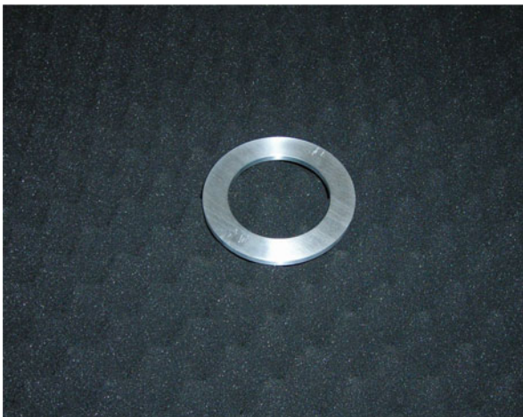
Fig. 6 Metallic ring used for the extended target reconstructions. Outer diameter: 126 mm, inner diameter: 84 mm. The one-dimensional sampling pattern consisted of two data sets of 40 points each. The separation between every point was \sim 1.6 mm ( 1/2 wavelength) and the separation between each data set was 105 mm. The data sets were separated from each other because of mechanical limitations imposed by the test bed design
