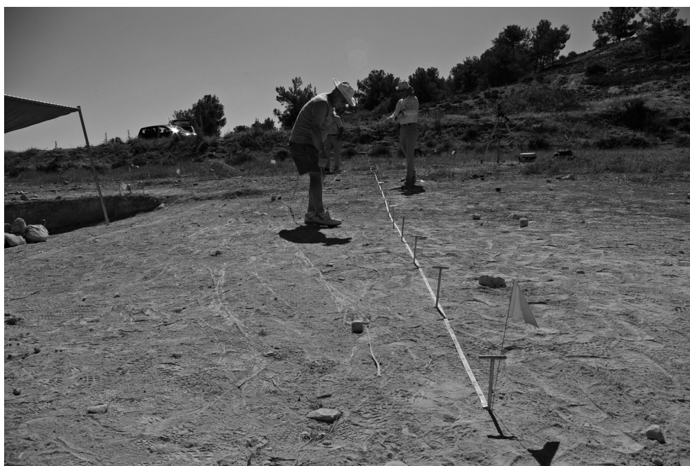
Fig. 12. John Hunt (foreground) and John Czarzasty (background) aligning an east-west Wenner array of probes for vertical soil resistivity survey south of Area X at Politiko- Troullia , 2008 (Photo by Sid Rempel).
