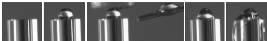
Fig. 3 Sealing method of the probe: gluing a 350\text{-}\mu\text{m} sphere to the tip of a 300\text{-}\mu\text{m} -inner-diameter HWG with UV-cured epoxy.
